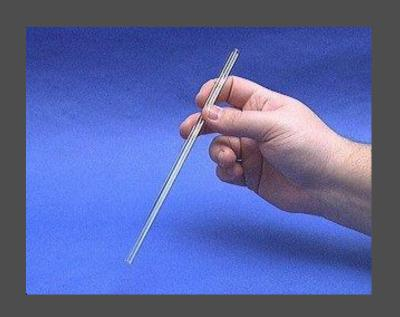
A glass rod is used to manually stir solutions. It can also be used to transfer a single drop of a solution.
