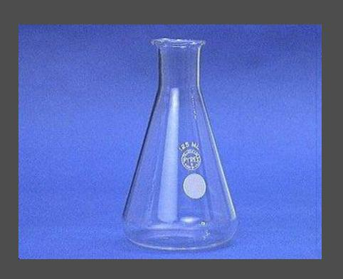
Erlenmeyer flasks hold solids or liquids that may release gases during a reaction or that are likely to splatter if stirred or heated.
