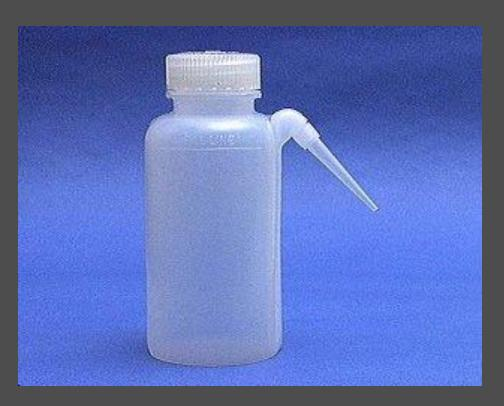
A wash bottle has a spout that delivers a wash solution to a specific area. Distilled water is the only liquid that should be used in a wash bottle.
