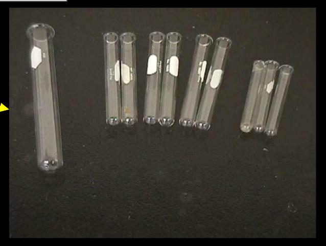
Used for reacting small quantities and for heating reactants
