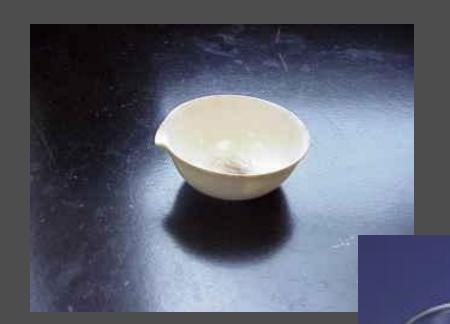
The evaporating dish is used for the heating of stable solid compounds and elements.
