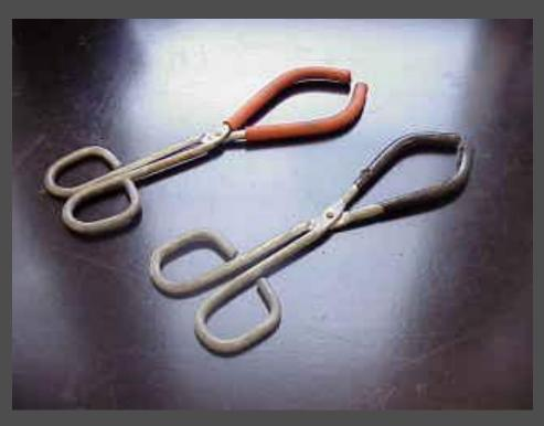
Beaker tongs are used to move beakers containing hot liquids
