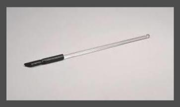
The attached rubberpoliceman is for transferring solids. Don't stir with this end!
